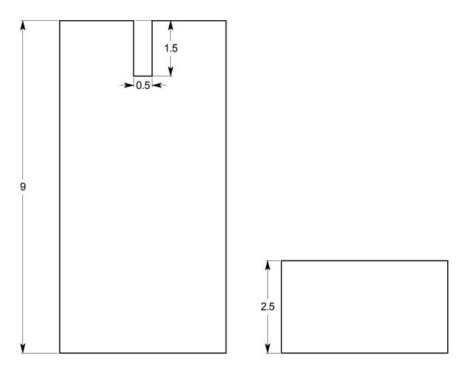
To cut the notch you can make several parallel saw cuts and chisel or drill out the bottom of the notch.
